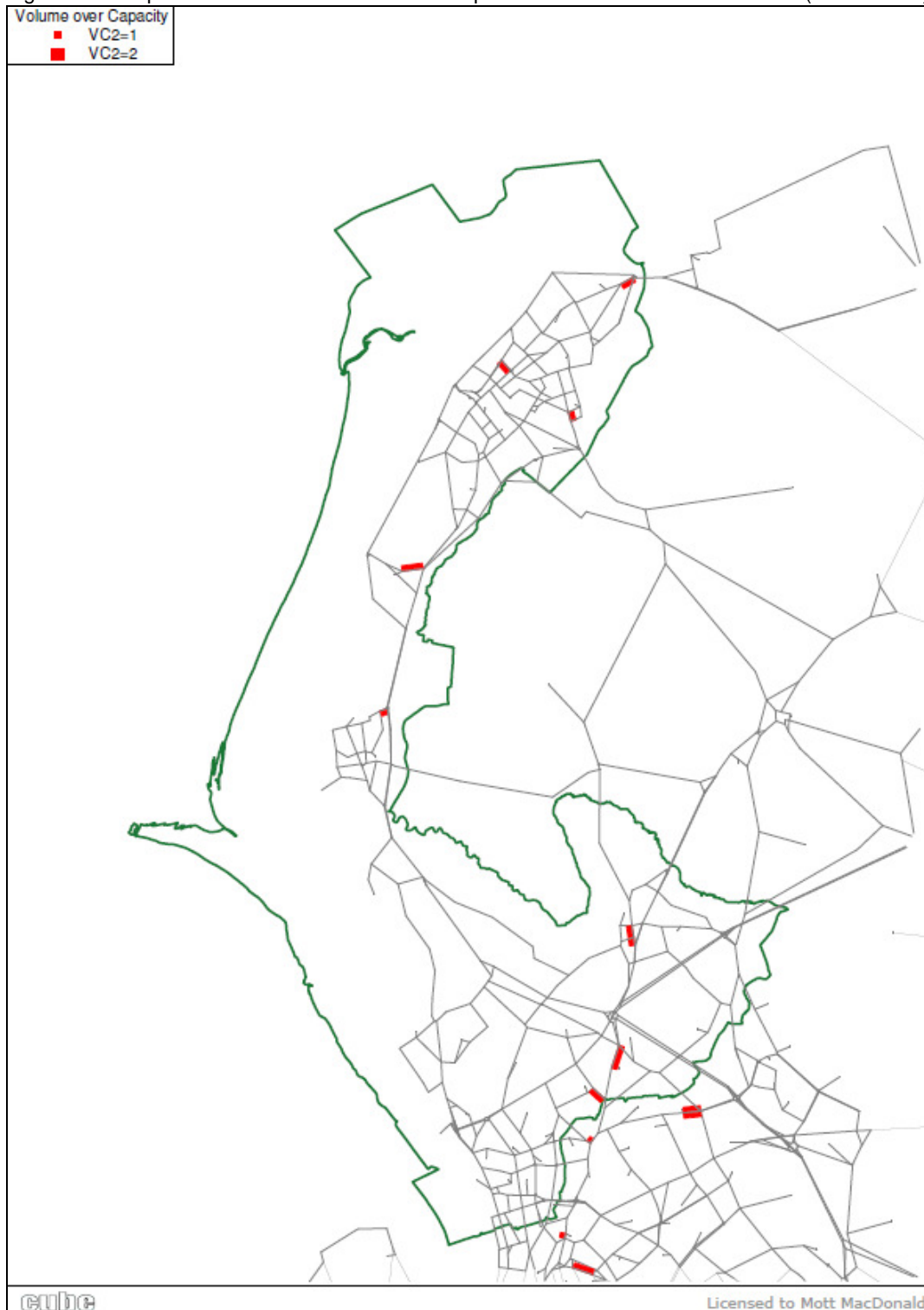
Figure D.1: Option 2 : V/C > 85% where V/C in Option 1 < 85% in the AM Peak Hour (08.00-09.00)
