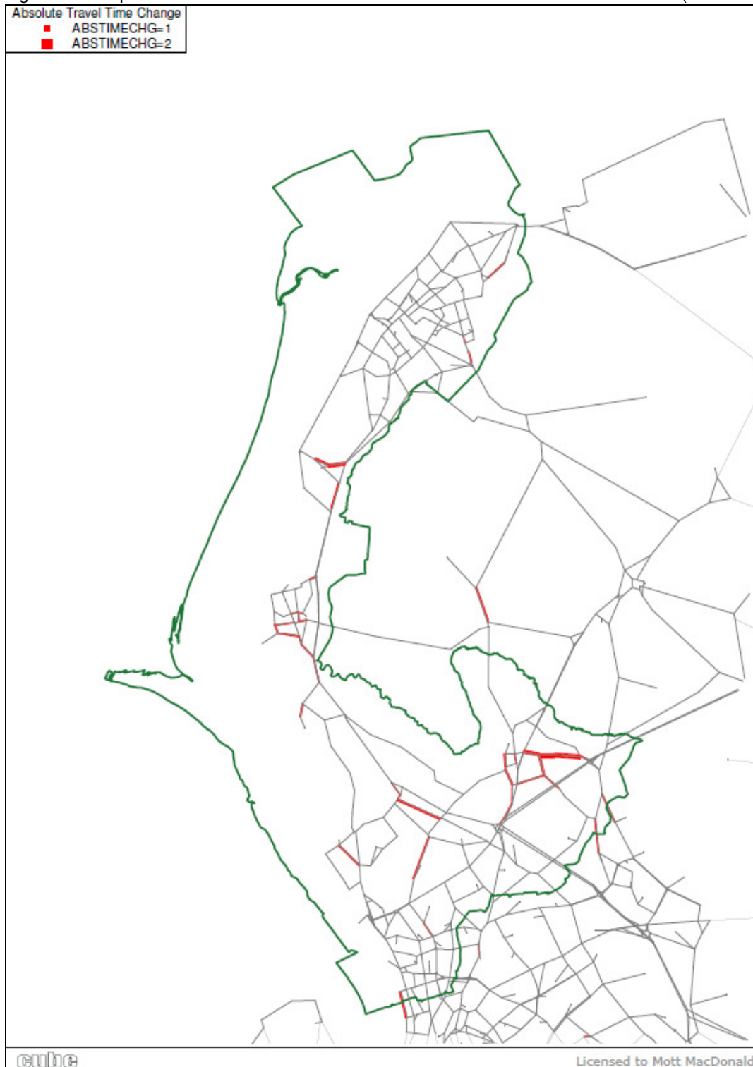
Figure E.4: Option 3 : Increase in Travel Time of Greater Than 5% in the PM Peak Hour (17.00-18.00)
