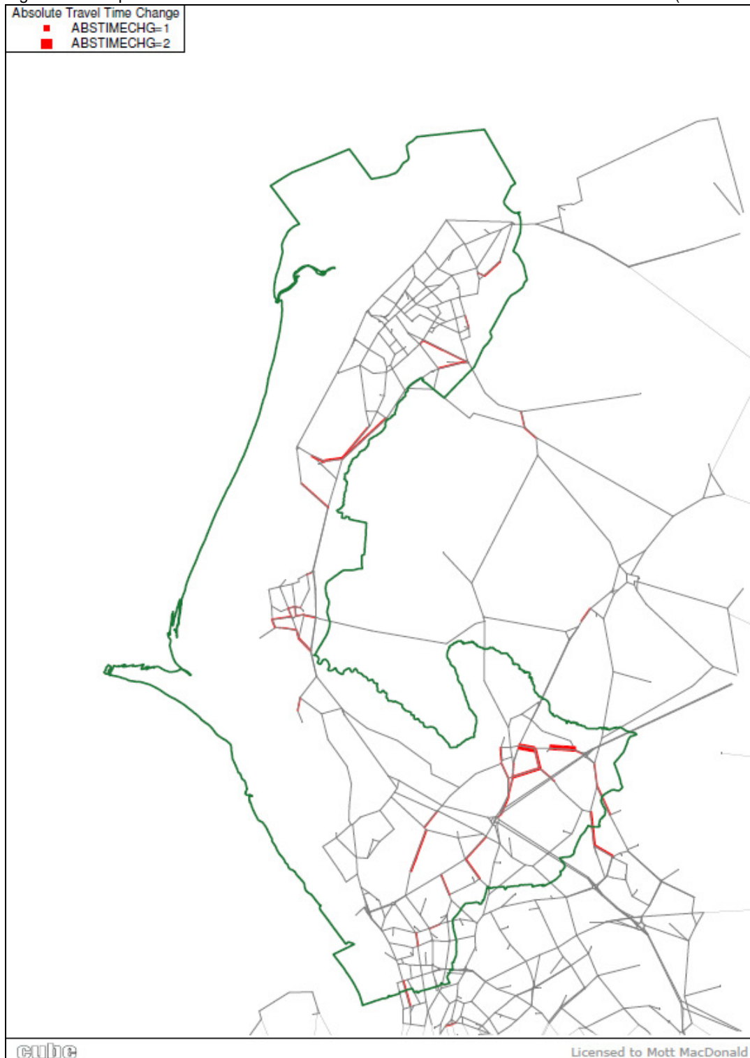
Figure E.3: Option 3 : Increase in Travel Time of Greater Than 5% in the AM Peak Hour (08.00-09.00)
