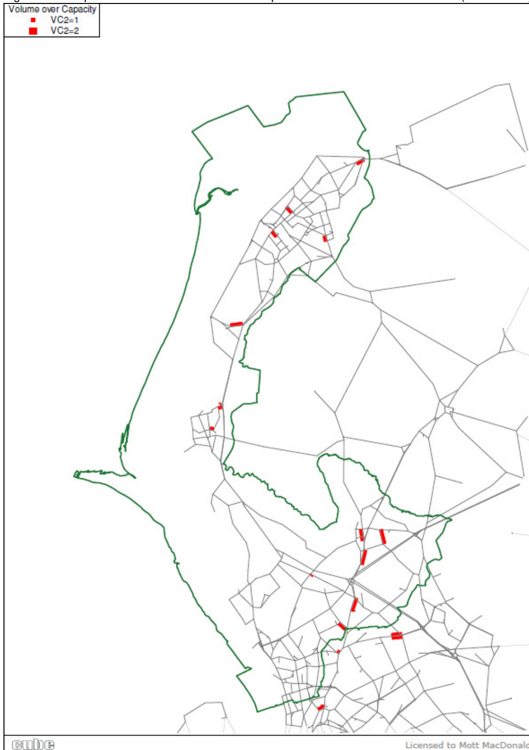
Figure D.3: Option 3 : V/C > 85% where V/C in Option 1 < 85% in the AM Peak Hour (08.00-09.00)
