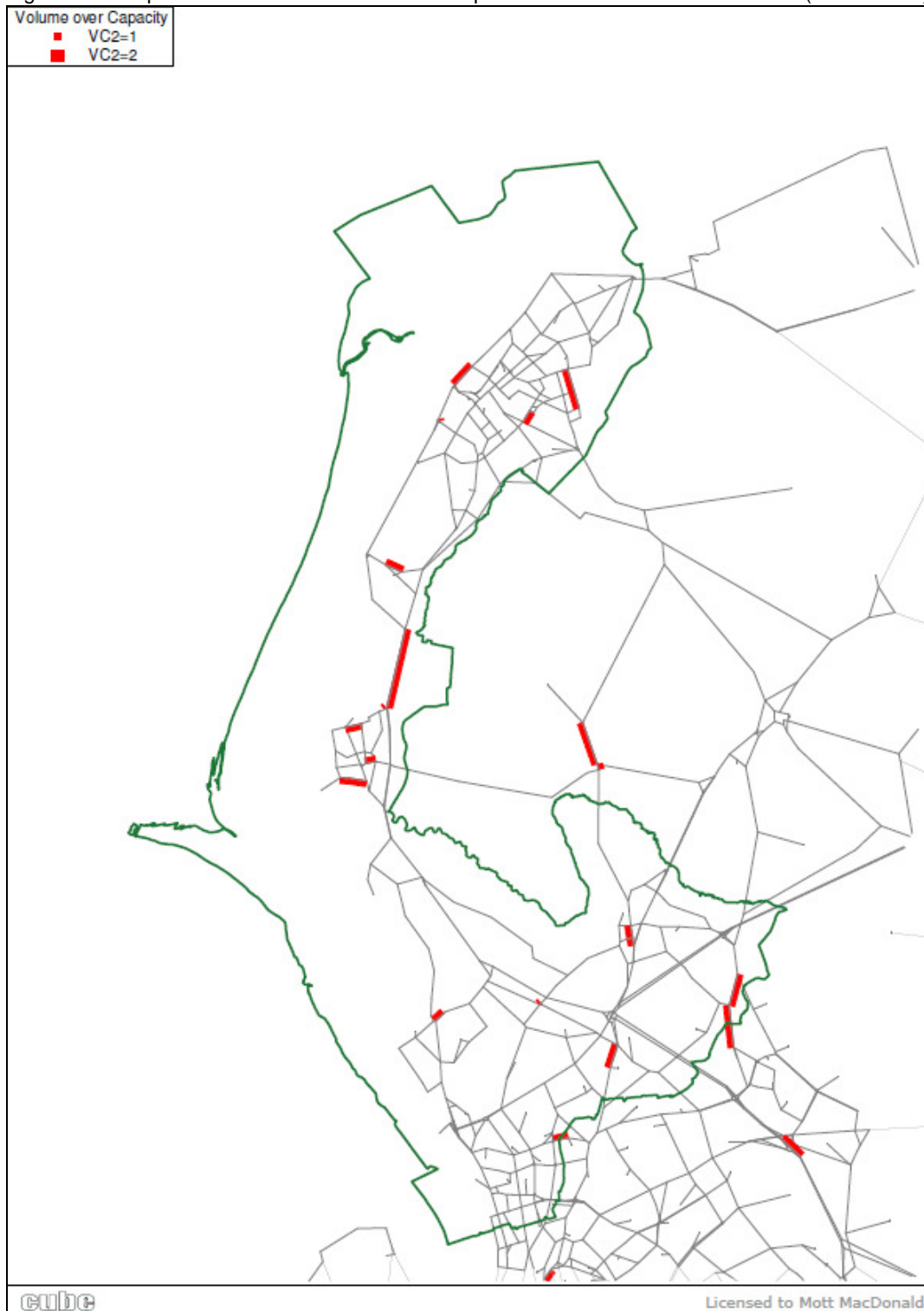
Figure D.4: Option 3 : V/C > 85% where V/C in Option 1 < 85% in the PM Peak Hour (17.00-18.00)
